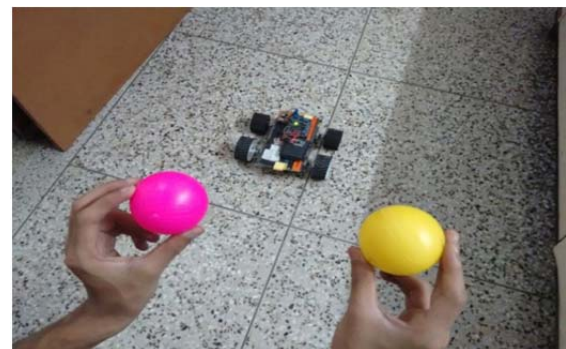
Fig. 8 The y co-ordinate of object1 is equal to the y co-ordinate of object2. Hence, the robot moves FORWARD
