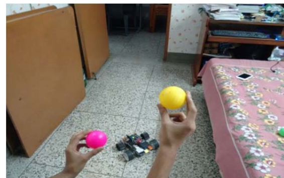
Fig. 10 The y co-ordinate of object1 is greater than the y co-ordinate of object2. Hence, the robot moves RIGHT
