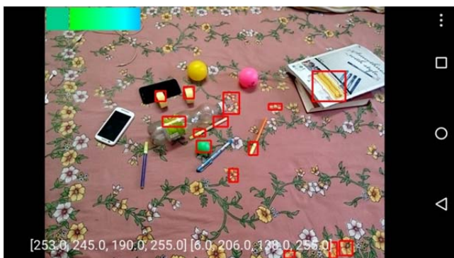
Fig. 3 The Application focuses on the given two RGB values once the “Start processing” button is pressed. In this case one of the RGB value is a shade of yellow and the other is a shade of green as marked by red rectangles.
