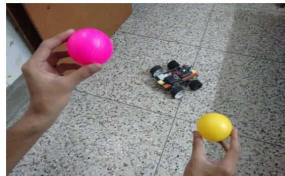
Fig. 9 The y co-ordinate of object1 is less than the y co-ordinate of object2. Hence, the robot moves LEFT
